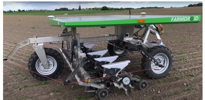
Robots in hoeing operation
